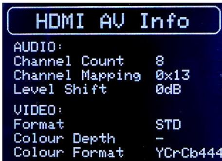
**Channel Count:** Indicated number of channels in the “Audio Channel Count” (CC bits). Value can range from 2 to 8.
