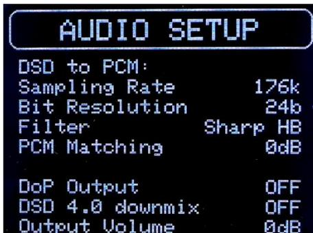
**Sampling Rate:** Sets the output sampling rate for DSD to PCM conversion. The options available are 88.2 and 176.4kHz.
