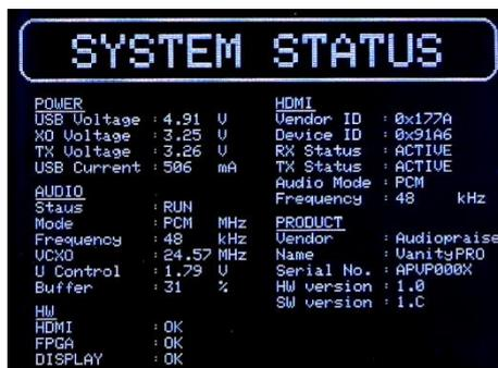
**POWER:** Shows internal voltage measurements of various voltage rails and Audio side power input current.
